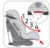
Release the safety lock (SR) of the safety bolt (SB) on the top of the back of the base (BT) and pull the safety bolt (SB) sideways out of the base holes (BL). Now the seat part (ST) is unlocked and can be clapped forward.
