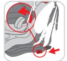
Release the safety bar (**SR**) of the safety bolt (**SB**) at the top of the back of the base (**BT**) and pull out the safety bolt (**SB**) sideways from the base holes (**BL**). Now the seat part (**ST**) is unlocked and will be clapped forward.
