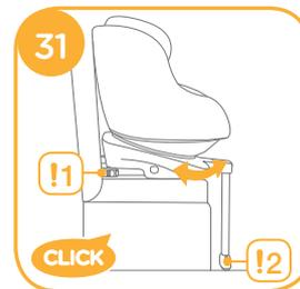
! The load leg must be installed correctly with green indicator. **31 -2**
