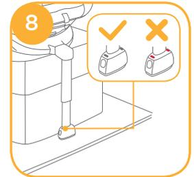
! Check to make sure the base is securely installed by pulling on both ISOFIX connectors.
