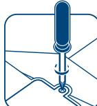
Make sure battery compartment is secure.
