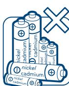
Do not use Nickel Cadmium rechargeable batteries.
