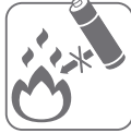
Never dispose of batteries in fire as this may cause them to explode.
