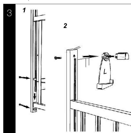
1) Attach the lower and middle rod supports, using 4 of the short bolts. Pass the rods through the side, middle supports, and into the lower support, as shown.
