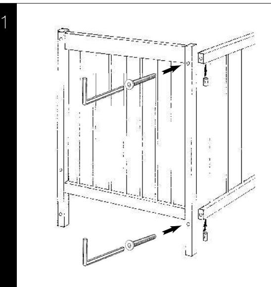
Attach the fixed side to the ends, using the long bolts and barrel nuts, as shown.
