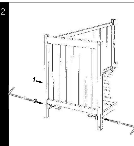
Attach the mattress base in the higher (1) or lower (2) position, using the medium bolts and base nuts, as shown. The lowest position is the safest (please see section 6: Safety Notes).
