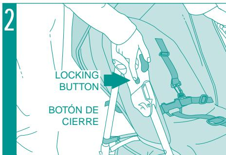
To fold the Three-wheeler press the locking button firmly and at the same time press both buttons on the front of the two side locks. Lift up the two handles, the Three-wheeler will fold.
